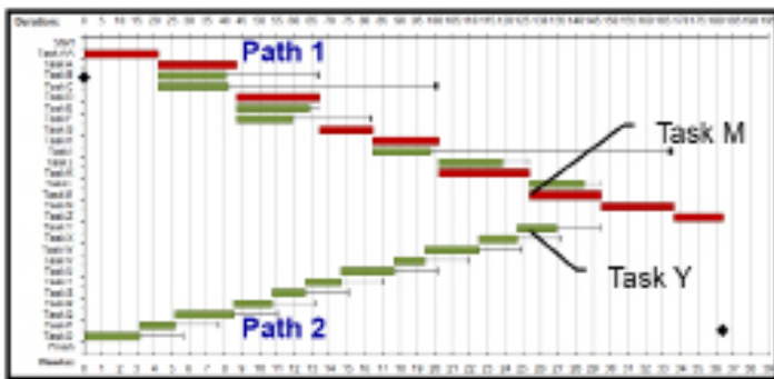
Figure 2. Critical Path for a Simple Network, Using CPM Calculations Only
