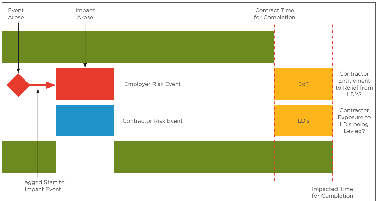
Figure 4. Example of the ‘Concurrent Effect’ of an Employer and Contractor Risk Event
