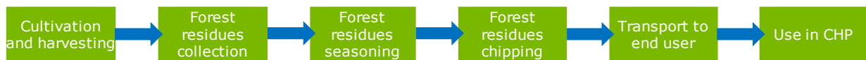
Figure 6. Example of pathway for the production of electricity and/or heat or cooling from forestry residues
