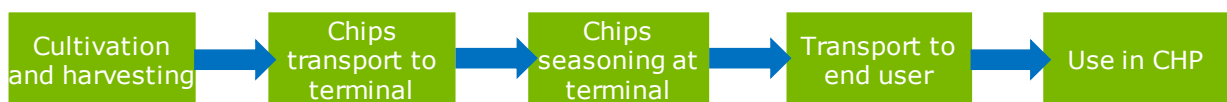
Figure 5. Example of pathway for the production of electricity and/or heat or cooling from virgin forestry
