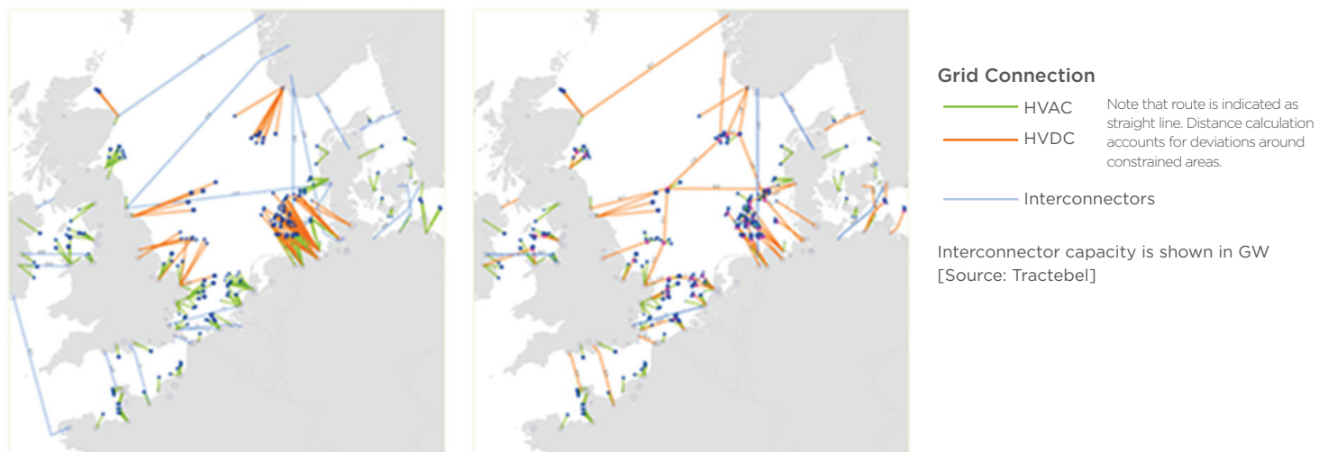
FIGURE 1: RADIAL (LEFT) AND MESHED (RIGHT) DESIGNS FOR A FUTURE NORTH SEA OFFSHORE GRID
